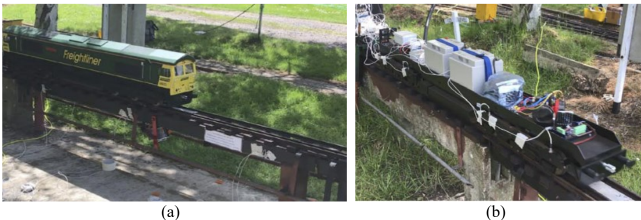
Figure 6 – Scaled model: (a) Train and bridge overview and (b) sensor placement. Adapted from (HAJIALIZADEH, 2022b).
